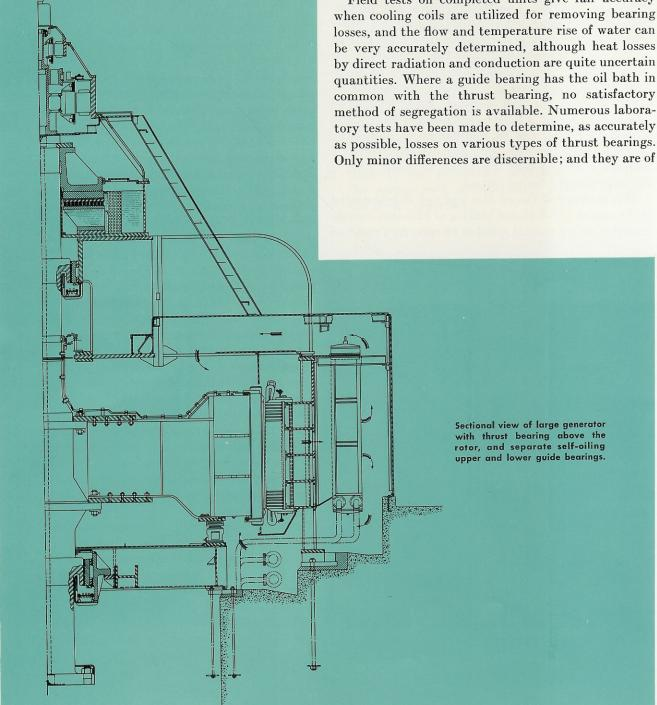
less significance than variations which accompany loading, temperature, and oil viscosity during operation. G-E thrust bearings are designed for loadings of approximately 400 to 600 pounds per square inch.
