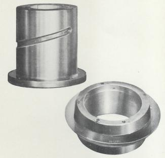
Thrust collar and guide bearing, showing oil grooves.
