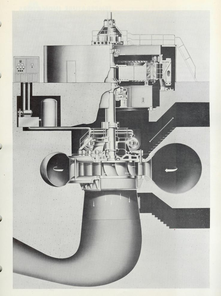
Alignment of the unit depends on the one generator guide bearing and the waterwheel guide bearing.
