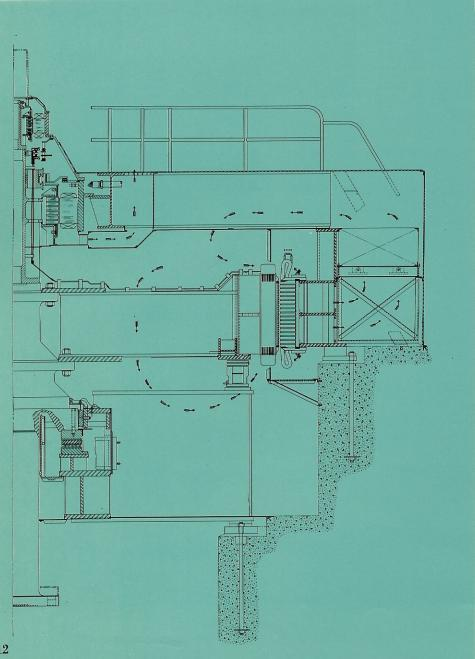
Sectional view of hydraulic turbinedriven generator with combined guide and thrust bearing below the rotor and without upper guide bearing.
