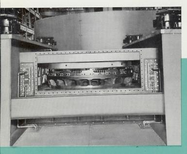
Lower bearing bracket showing bearing base ring, spring cage, springs, babbitted segments and runner in position in bearing housing of large unit.
